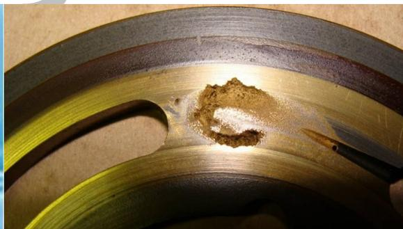
Damaged surface due to implosion
